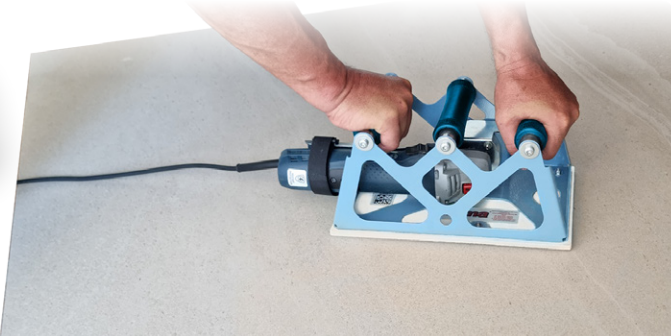
Electric Vibrating Tile Beater with universal attachment for angle grinders from 700 to 1400 W. Perfect for beating tiles and waterproof membrane , allows the correct expulsion of air . Using a angle grinder with variable speed , the vibration intensity can be adjusted as required. Equipped with an Anti-Mark base with vibrating area 30x19cm and ergonomic handles. Easy to handle with low weight (3 kg without grinder). *grinder not included
